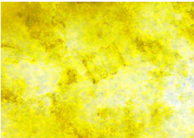
I would conclude that the cornflakes are the product of organic matter decomposing as calcite also deposits in the pipes. Photosystems were likely still running for a few days in the thylakoids of the algal plastids as they died in the pipes, and this activity would deposit calcite by continuing to alkalize the aqueous solutions, in large part by depleting CO<sub>2</sub>.
