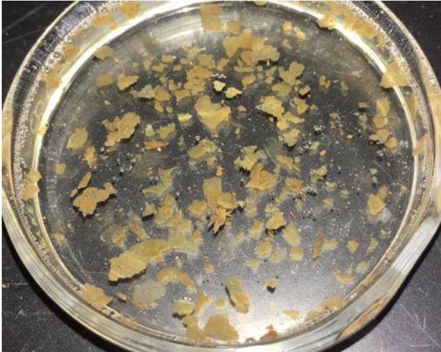
The acid bath (24 hours) did not dissolve/react all material. Micrographs from what was left behind showed a lot of organic matter, which held the flakes together despite the long-term saturation. Some bodies of algae, both greens and possibly golds, could be seen.
