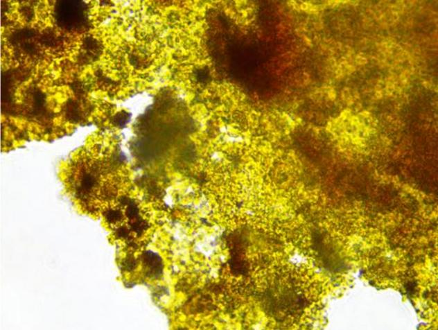
An acid bath (5% acetic acid) showed strong effervescence, suggesting a calcium-rich matrix is holding the chemically mixed material together.
